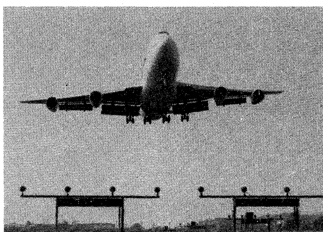
Fig. 1 747-JT9D (RA001) aircraft with high lift devices and landing gear deployed during approach.
